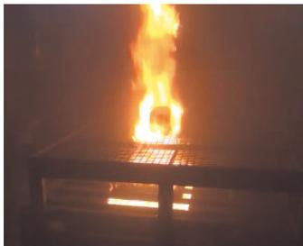
External short circuit protection 外部短絡
