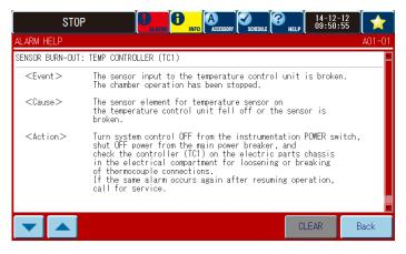
3) See "6.1.2 List of alarms", and then take the actions that correspond to the error contents shown on the instrumentation display.
