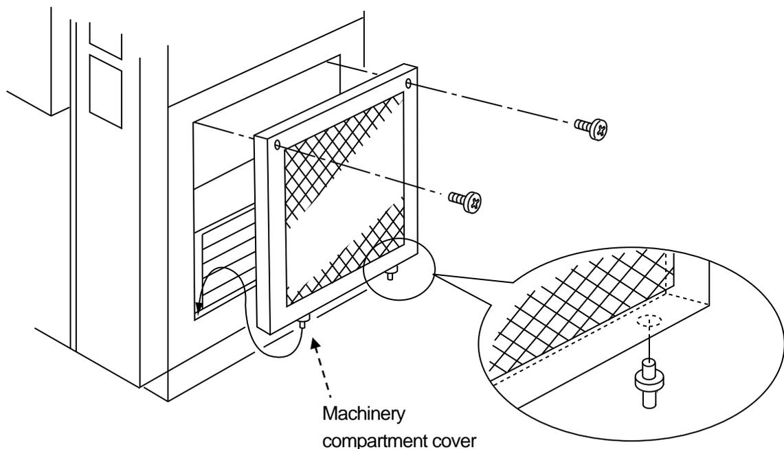
Two pins are installed along the bottom of the cover.
