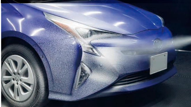
Snow adhesion test
