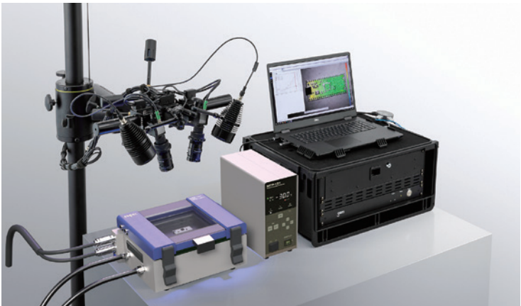
Temperature-Dependent Warpage Measurement System 3D DIC + One-Device Temperature Test Chamber
