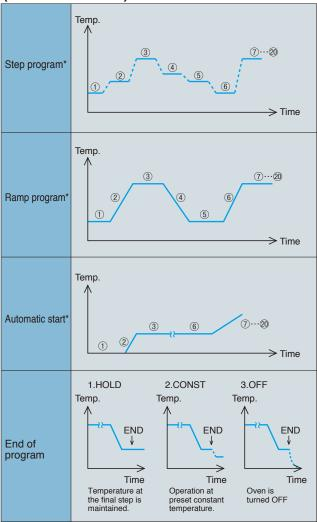
$_{\mbox{\tiny \#}}$  The number of repetitions of a program can be preset between 1 and 999. Stepwise damper setting is possible.
