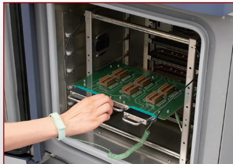
DUT board with shorting connectors
