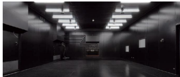
Test chamber: Width 6 m x Depth 9 m x Height 3 m A black coating is applied to suppress the diffuse reflection of light.
