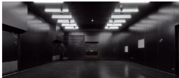
Test chamber: Width 6 m x Depth 9 m x Height 3 m
