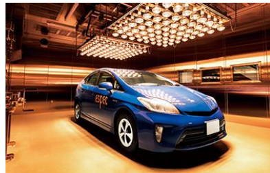
Drive-In Chamber for Vehicle Testing
