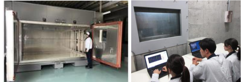
Capable of performing various safety tests for secondary batteries compliant with United Nations regulations and other standards
