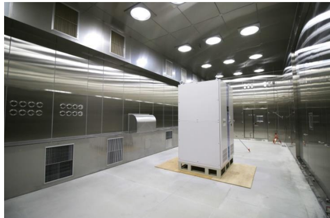
Large Walk-in Type Temperature & Humidity Chamber
