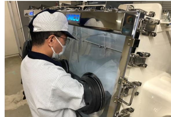
Glovebox for dismantling cells
