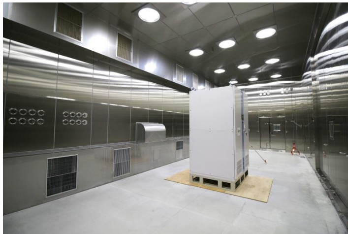
Large Walk-in Type Temperature & Humidity Chamber
