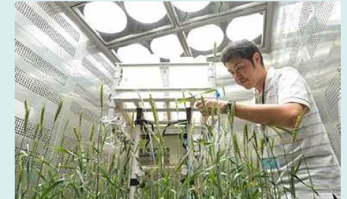
Experimental System for Analyzing Responses of Dryland Plants to Climate Change (Arid Land Research Center, Tottori University)
