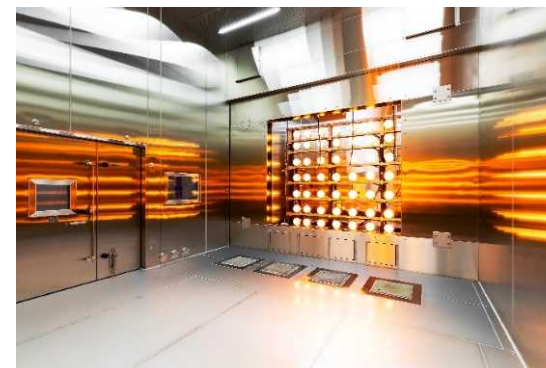
Furnished with irradiation equipment and watering (rain) equipment, to reproduce an outdoor weather environment
