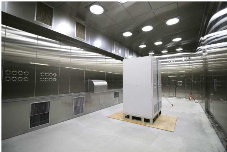
Large Walk-in Type Temperature & Humidity Chamber
