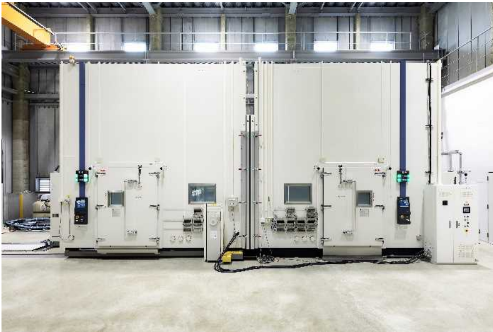
Walk-in Type Temperature (& Humidity) Chambers, for use for building materials
