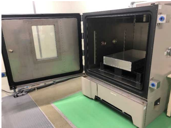
Pack battery low-temperature dismantling chamber
