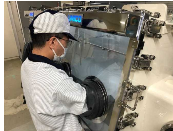
Glovebox for dismantling cells
