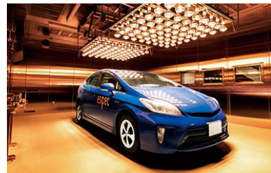
Drive-In Chamber for Vehicle Testing
