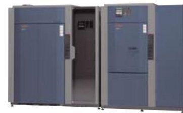
Burn-In chamber for semiconductor inspection
