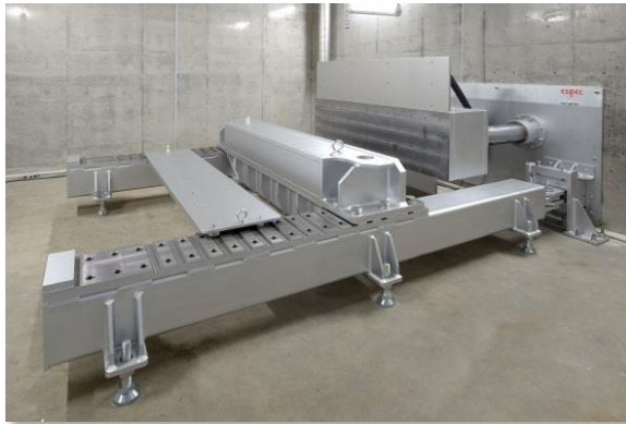
Crush Testing Equipment (No. 1 Safety Test Room)
