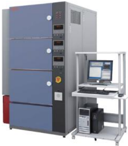
Charge-discharge Cycle Evaluation Equipment
