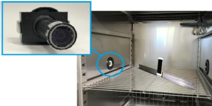
Image of in-chamber monitoring camera
