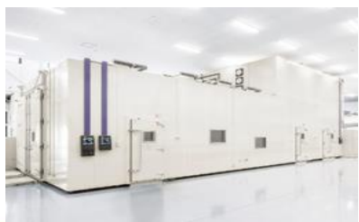
Top left: Testing in snow conditions Top right: Testing in fog conditions Left: Exterior of All Weather Simulation Chamber
