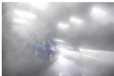
Top left: Testing in snow conditions Top right: Testing in fog conditions Left: Exterior of All Weather Simulation Chamber
