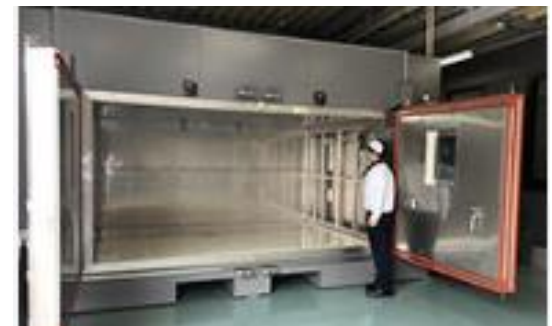
Large temperature cycle testing system (Battery Safety Testing Center)
