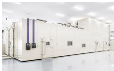
Top left: Testing in snow conditions Top right: Testing in fog conditions Left: Exterior of all weather simulation chamber
