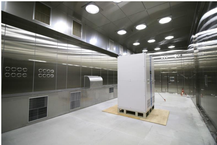
Large walk-in type temperature & humidity chamber
