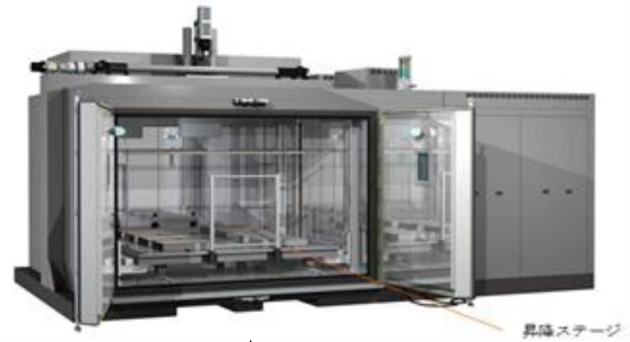
Nail penetration/crush testing equipment Capable of handling cells and battery packs
