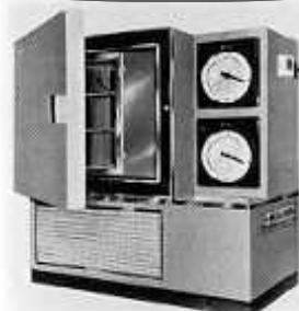
Low temperature & humidity chamber "Lucifer" (1961)
