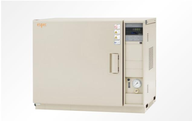
The built-in inert-gas sealing system allows the chamber to be filled with an inert gas such as CO<sub>2</sub> or N<sub>2</sub> for anaerobic heat treatment or temperature characteristics testing. An optional O<sub>2</sub> concentration indicator controller equipped with an oxygen sensor is available (for N<sub>2</sub> gas only)
