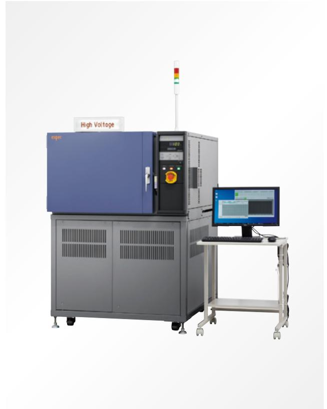
The High-Temperature Reverse Bias Test System measures and evaluates leakage current behavior under high-temperature, high-voltage stress conditions as a time-lapse breakdown test of power semiconductor insulation films. With a gate-off voltage applied to the gate terminals of power semiconductors such as IGBTs and power MOSFETs, a reverse bias of several hundreds to 3 kV is applied as a stress voltage across D-S, and  $I_{ce}$  /  $I_{ds}$  leakage current is measured and logged periodically.
