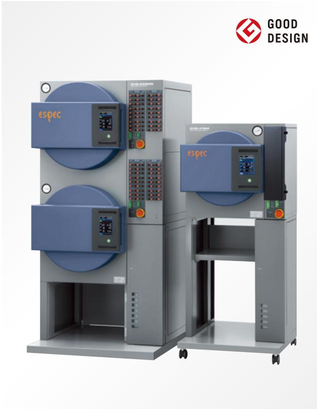
HAST system offers highly precise moisture absorption conditions and short test hours, attracting attention as a method of evaluating and analyzing moisture resistance. Two control functions: the M type with wet and dry bulb temperature control, unsaturated control, and wet saturated control, and the Standard type with unsaturated control and wet saturated control. The M type conforms to IEC60068-2-66. For the 2-stage type, test condition for each unit can be set and operated individually.
