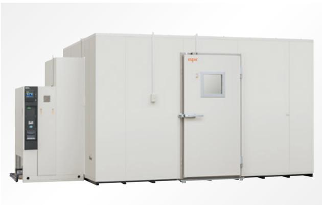
Suitable for long storage in medical, cosmetic, and food industries. It adopts "area temperature & humidity control," which is to control test area's environment by detecting difference between setting and measured values. Thanks to it, high-precision temperature and humidity distribution is realized;  $\pm 1^{\circ}\text{C}$   $\pm 5\%$ rh as maximum gap in test area is guaranteed.
