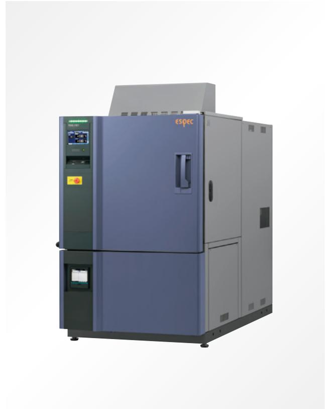
This chamber enables rapid specimen temperature changes, covering a wide range of applications from JEDEC and IEC tests standard to screening. The chamber applies uniform temperature stress to specimens with excellent temperature distribution performance. Two control modes offered: Temperature Ramp Control mode that enables ramp control at a specimen temperature change rate of 15°C/min, and Air Temperature Non-ramp Control mode that enables temperature cycle testing and thermal shock testing.
