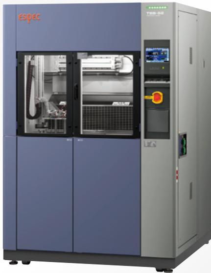
Liquid-to-liquid thermal shock chamber capable of imposing higher stress on the samples. Of a small required footprint, the high degree of airtightness in the test area and the numerous mechanisms developed allow reducing brine consumption and therefore, running costs.
