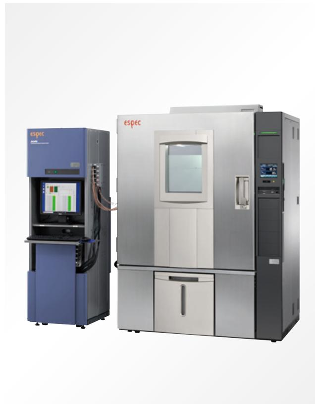
The THB Evaluation System conducts a reliability test for LSI such as automotive semiconductors which require higher reliability under rigorous conditions than consumer semiconductors.
