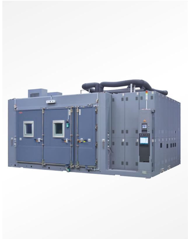
The chamber allows a thermal cycle between the temperature range of -180°C to +170°C. Adopting a conventional and LN<sub>2</sub> hybrid cooling system realizes low running cost while achieving high-precision control throughout the range.
