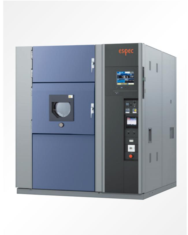
The hot chamber at the top of the thermal shock chamber (TSA) has been changed to a high temperature and humidity chamber that can control humidity, thereby enabling dew cycle tests. The ability to perform two tests in one unit not only lowers costs and space requirements, but it also saves on the labor required to insert and remove specimens, thereby reducing testing workforce.
