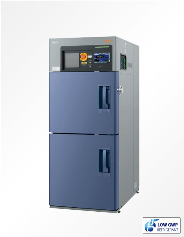
A temperature recovery time of less than 5 minutes is achieved in 2 zones (+150°C and -65°C) without auxiliary cooling. Complies with MIL-STD-883 and other test standards.
