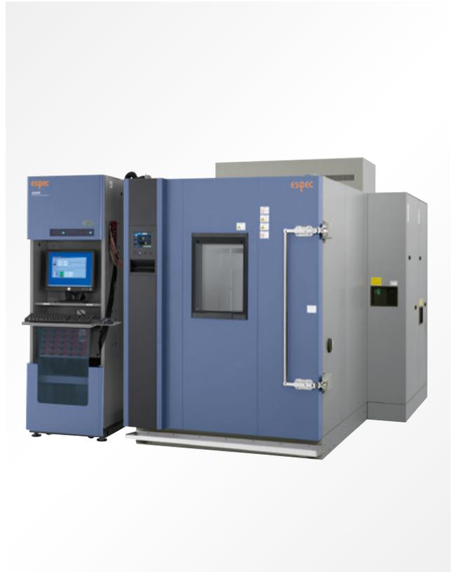
The PV Module Thermal Cycling (TC) Test System combines a large capacity temperature and humidity chamber, which is equipped with a jig to securely hold multiple PV modules, and with safety of operators in mind, and a current load measurement system, which applies a current, that is equivalent to STC peak output current, controls the entire system, thereby enabling easy thermal cycling (TC) testing.
