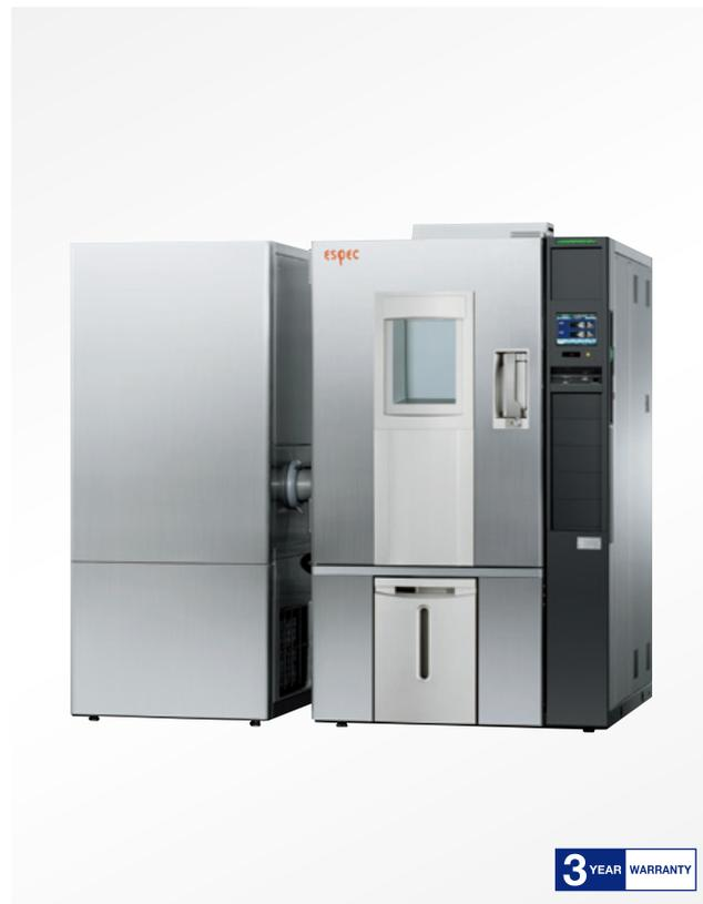
A rotary regenerating (adsorption) dehumidification system ensures accurate low humidity tests at low temperatures from +10°C / 15%rh to +20°C / 10%rh, suitable for electrostatic reliability tests. Continuous long operation of 500 hours is possible throughout the entire range of low humidity.
