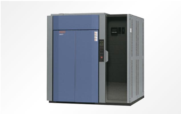
Temperature and various electrical stresses are applied to semiconductor devices and assembled electronics, which is valid for screening semiconductor devices with surface contamination and input circuit deterioration. With our original air conditioning system, it can match the heat dissipation and maintain the temperature conditions during the process. It comes in two types: A1 exclusively for static burn-in; and B1 which can be modified to a clock burn-in system.
