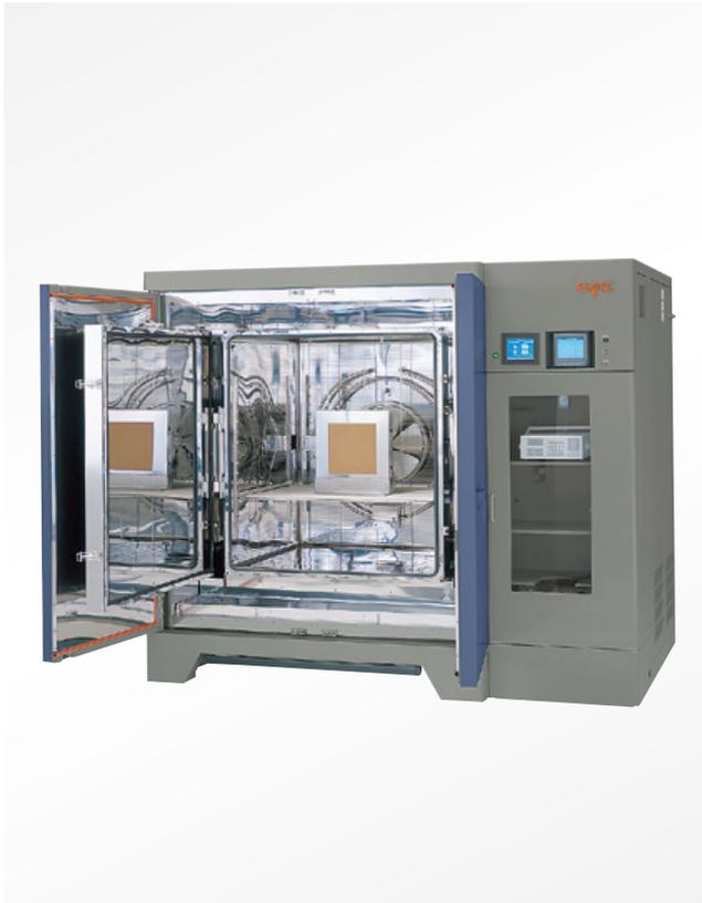
Volatile organic compounds (VOC) is known to cause sick building syndrome or SBS. ESPEC has developed a VOC chamber that can be used to capture VOC given off by construction materials such as plywood, wallpapers, and curtains, automotive components, PCs and other heat-generating equipment common to the household.
