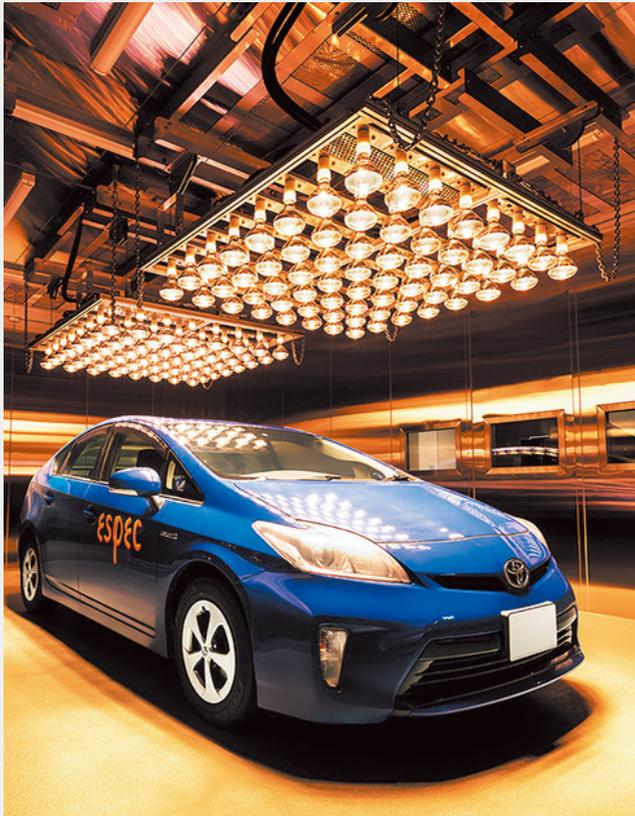
Walk-in type temperature and humidity chamber with insulation device for full-scale vehicle testing. When a black panel is set in the section of the vehicle for temperature control, the reading of the temperature sensor attached to the black panel is fed back into the device to control the infrared lamps, enabling the intended temperature to be set in the vehicle's location (black panel)
