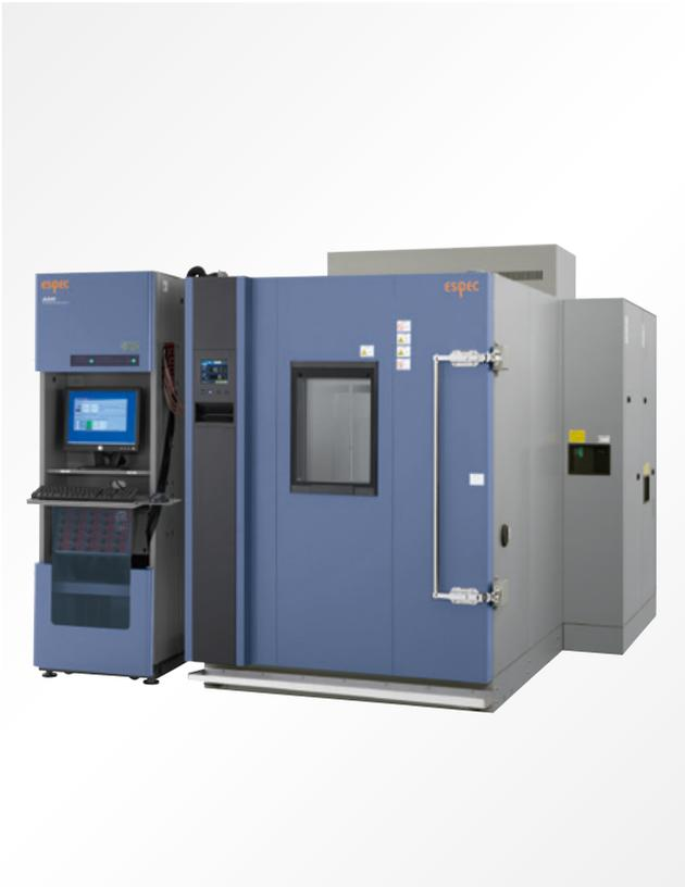
Potential Induced Degradation (PID) is an undesirable property of crystalline PV modules. It can occur when the voltage potential of the module and the leakage current drive ion mobility within the module between the semiconductor material and other elements of the module (e.g. glass, mount and frame) causes the power output capacity of the module to degrade.
