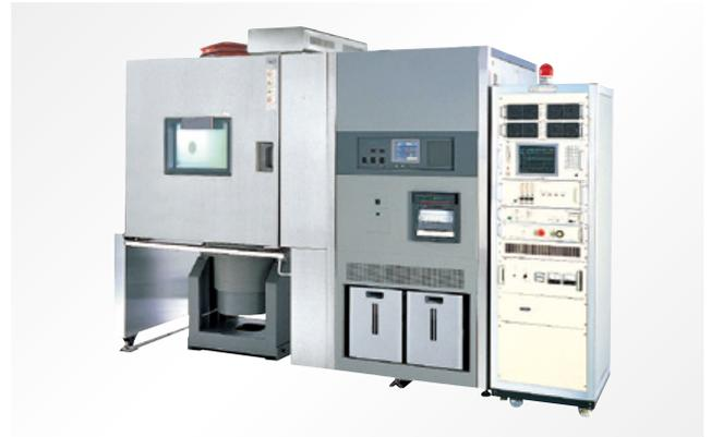
Simulates combinations of physical (mechanical) stress such as vibration, shock and acceleration in addition to environmental stress such as temperature and humidity.
