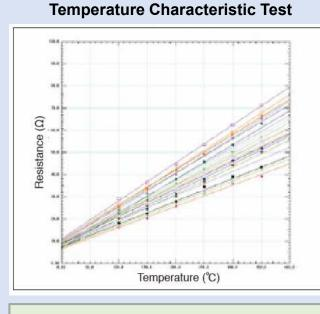
Display measured resistance per channel (sample)
