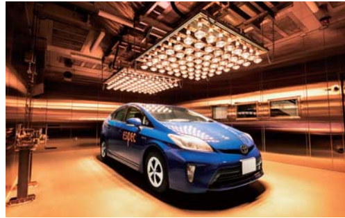
Drive-In Chamber for Vehicle Testing
