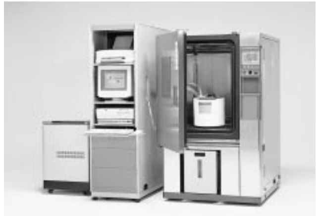
Photo 4 Weather-Proof Vibration Shaker (left), Connector short interruption evaluation system (center), and temperature and humidity chamber (right)
