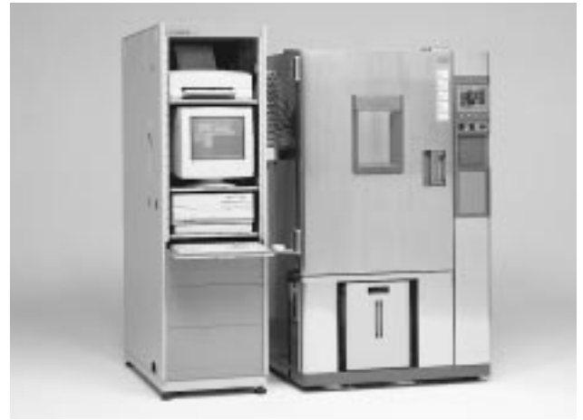
Photo 2 Ion Migration Evaluation System AMI-025-P (left), and Temperature and Humidity Chamber (right)
