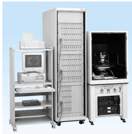
Photo 1 TDDB evaluation system (Espec model AMM-1000)
