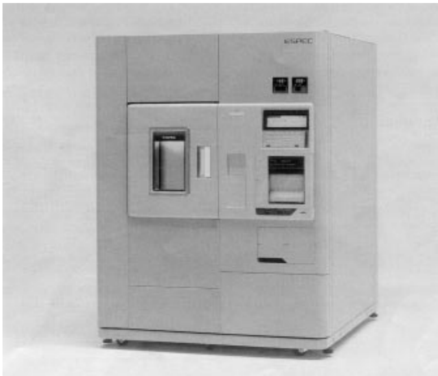
Photo 2 Dew cycle test chamber produced at Tabai Espac
