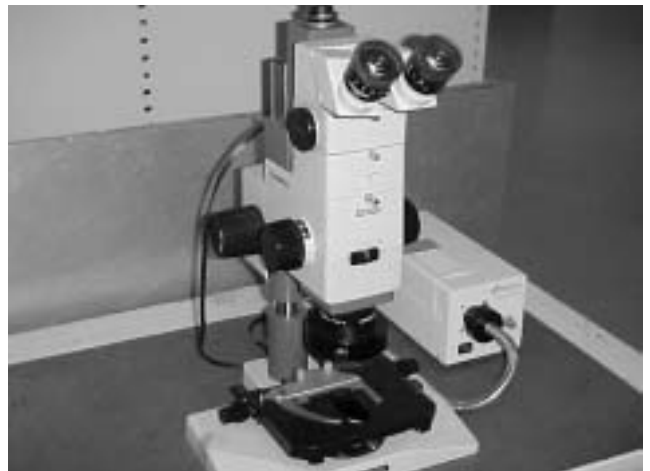
Photo 1 Detecting points for analysis (stereoscopic microscope)
