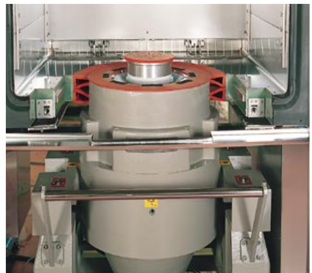
Photo. 9 Vibration generator connected to temperature/humidity chamber
