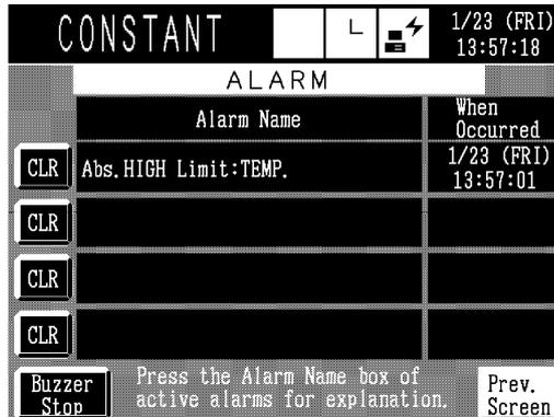
2. Press the  key to deactivate control power. Check the alarm table. If there is no need to shut OFF primary power supply, leave the main power switch in the ON position.
