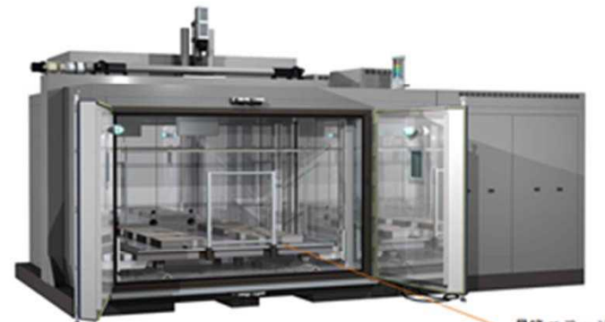
Nail penetration/crush testing equipment Capable of handling cells and battery packs
