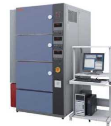
charge-discharge cycle evaluation equipment
