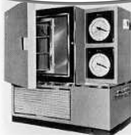
Low temperature & humidity chamber "Lucifer" (1961)
