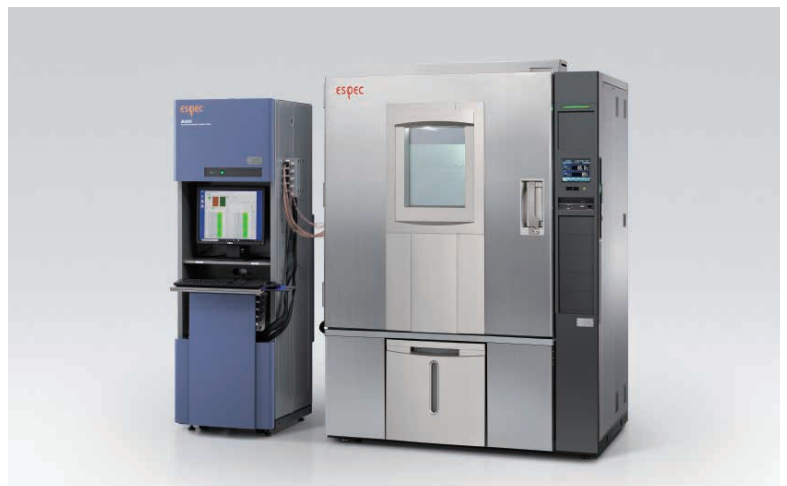
System integration with Electro-chemical Migration Evaluation System (example)
